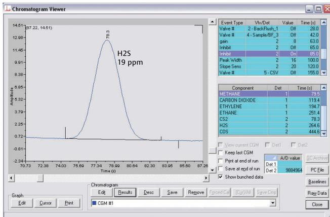
For many part-per-million applications, a simple, easy-to-maintain TCD detector can be used rather than a more complicated FID or FPD due to the superior sensitivity of the Rosemount Analytical TCD design.
